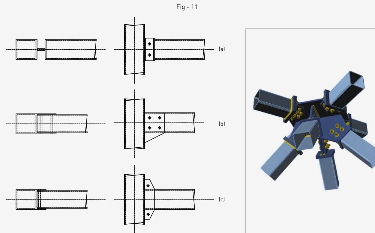
Typical connection of an RHS beam to an RHS column a,b&c
