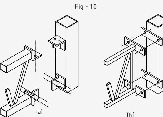
Figure 10(a&b) - Truss to SHS/RHS column connection
